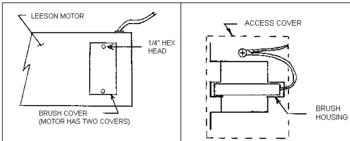
Motor brushes need periodic inspection and replacement as wear indicates. Brush wear is greatly influenced by individual application, voltage and heat load. It is recommended that brush wear be checked at early intervals of operation in order to determine future required inspection.
