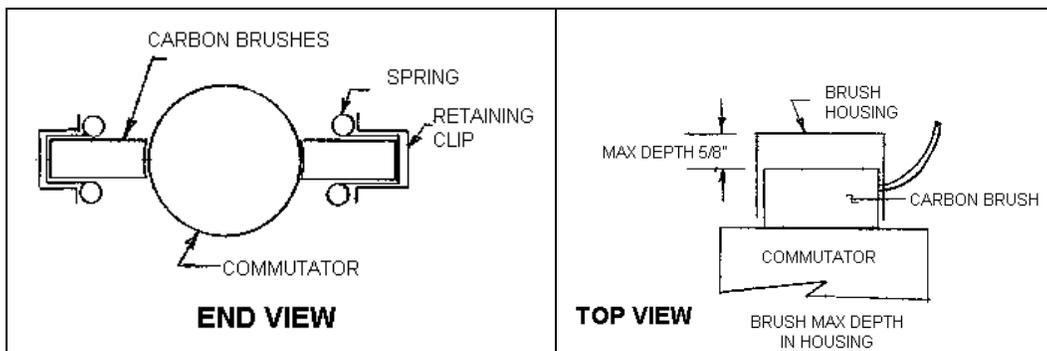
**Tip:** In a new motor with new brushes the back of the brush will be flush with the brush housing, as the brush wears the distance into the housing will increase. (See top view drawing below.) A quick measurement of the depth will be sufficient. When the brush is 5/8" into the holder it will need replacement. If in doubt change the brushes. Carry spares.
