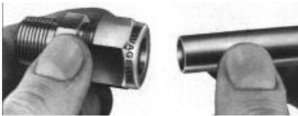
Figure 3 ~ Insert Tube into Fitting Body
