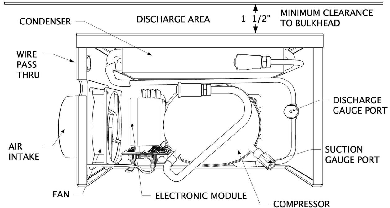
**An un-ducted unit in a poorly ventilated small space will run hot, lowering the cooling capacity, increasing power consumption, and possibly causing damage by overheating the compressor.**
